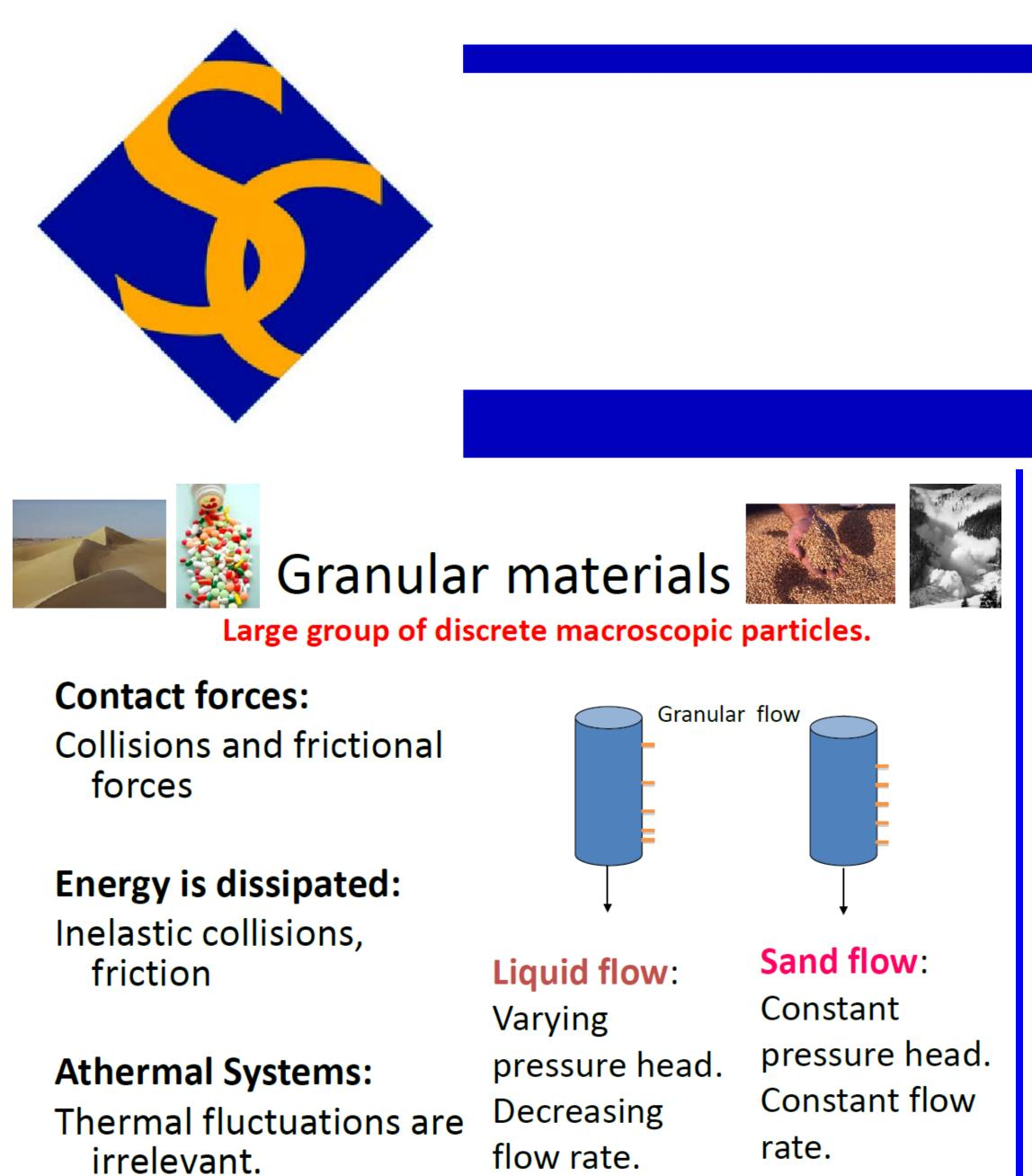
Measurement of Flow Rate
